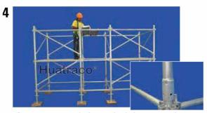
Set up temporary platforms, check the contact of vertical posts/standards using the sighting device provided on each triangle sleeve. The upper and lower tubes should be in contact at each leg.
